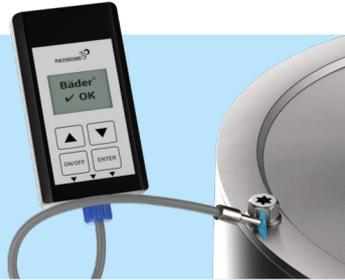
The security level Topsecure (BäderIdent®) offers an unambiguous product identification, making it an effective means against product counterfeiting and manipulation of every kind. The BäderIdent® lacquer system contains an individual code which consists of a specific fluorescent marker particle and a color. By means of a suitable analyser, you can always check on site the authenticity and integrity of your product.
