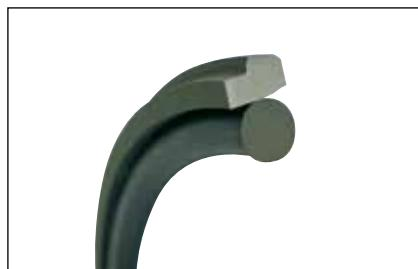
The Stepseal® 2K is a single-acting sealing element consisting of a sealing ring made of high-quality Turcon® or Zurcon® materials and an O-ring as an elastic pre-tensioning element.
