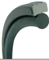
The Zurcon® Wynseal is a dual-acting piston seal, consisting of a special PU sealing ring with an O-ring as an elastic pre-tensioning element.
