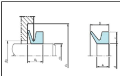
The V-ring is an axial lip seal for shafts and bearing sealing. The V-ring is mounted directly on the shaft and lies against a mating surface, e.g. the machine case. The V-ring provides reliable protection with low friction.
