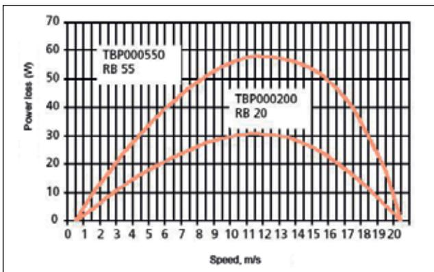
Power loss dependent on the circumferential speed, running surface made of steel, surface roughness 1.5–2.0  $\mu\text{m}$  Ra. Axial seal without lubrication.
