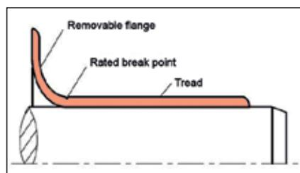
Design of the shaft protection sleeve
