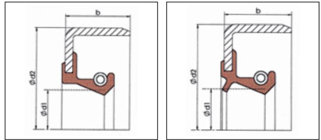
The outer surface of the case for types B and BS is metallic. Due to the lower elastomer content, the type B is particularly suitable for expensive materials; or for installation conditions which do not rule out damage to the soft rubber outer cover of the type A or AS.
