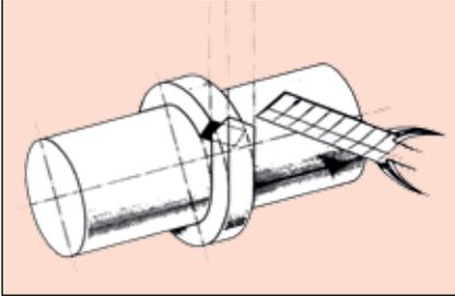
Open the rings in the axial direction, insert base ring and tighten slightly to give the exact form to the packing ring. Insert the second ring so that the incision is offset by 90°. Tighten slightly in order to install the other rings using the same method. The gland is permitted to enter maximum 1/3 of its free length (otherwise install another ring). When the shaft is rotating, completely release the gland and tighten again slightly.
