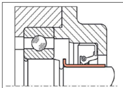
Running surface with shaft protection sleeve
