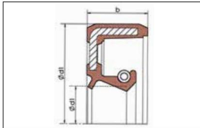
Radial shaft sealing rings are used for sealing rotating or pivoting shafts and axes.
