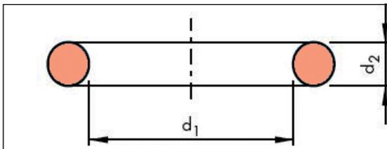
The O-ring is an endless manufactured round ring with circular cross section made of rubber-elastic materials.
