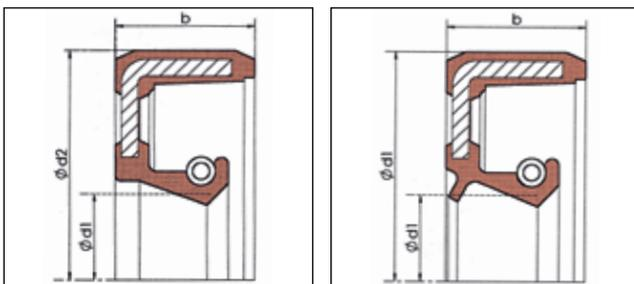
The outer surface of the types A and AS reinforcing ring has an elastomer cover which guarantees faultless leak tightness between the radial shaft sealing ring and the accommodating case hole, even for split cases and those made of materials with greater thermal expansion.
