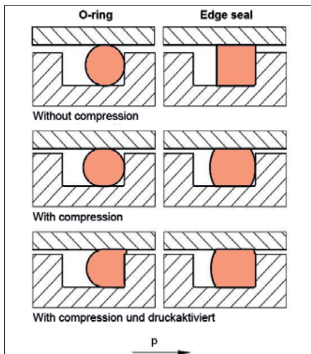
O-ring / edge seal installation comparison
