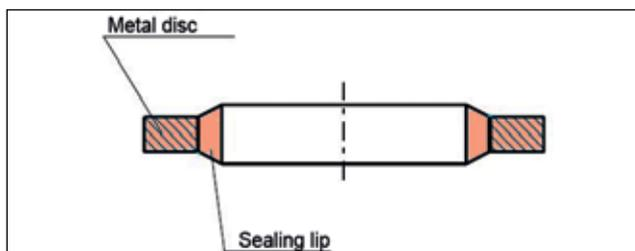
U-Seal sealing ring Standard SDS
