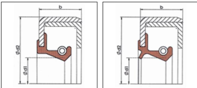
The types C and CS with metallic case and cap on the front side are manufactured on the outer surface like the types B and BS. The advantage of the large radial stiffness is mainly utilised for harsh installation conditions.
