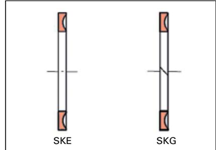
Thrust rings with concave cross section on one side
