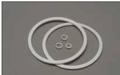
Thrust rings are protection and support elements made of extrusion-resistant materials; thrust rings are installed in a groove together with an elastomer seal - preferably with an O-ring or an X-ring seal. Due to the tight borehole cap, thrust rings prevent the extrusion of the pressurised elastomer sealing element into the sealing gap.
