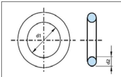
The O-ring is an endless pressed round ring with circular cross section made of rubber-elastic materials. O-rings are used both for static as well as for dynamic sealing in pneumatics and hydraulics.
