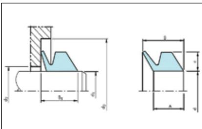
The V-ring is an axial lip seal for shafts and bearing sealing. The V-ring is mounted directly on the shaft and lies against a mating surface, e.g. the machine case. The V-ring provides reliable protection with low friction. Design with a diagonal on the back side.
