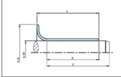
The shaft protection sleeve is used as running surface for radial shaft sealing rings. It consists of a thin-walled, cylindrical pipe with a mounting flange.
