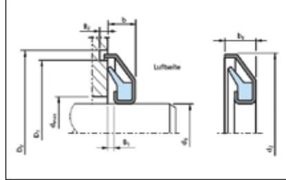
The Gamma ring consists of an elastic sealing collar and a metal case. It is mainly used for sealing from external contaminants, liquid sprayers, grease etc.
