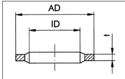
Screw seals are gaskets – a washer with vulcanised sealing lip. They are used for static sealing of screw connections and fastening elements. The screw seal is distinguished by easy to use and an inexpensive solution in operation.
