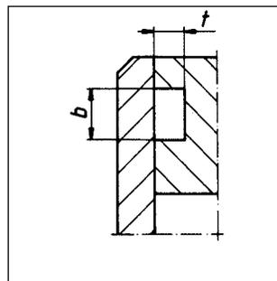
The groove dimensions  $t$  and  $b$  are dependent on the cord diameter  $d_2$ .
