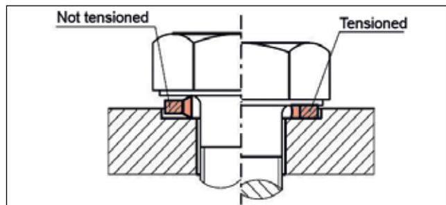
U-Seal sealing ring Standard SDS
