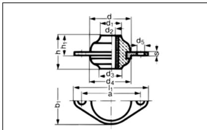
For tensile and pressure load and high safety requirements. Special design without the usual bonding methods:
