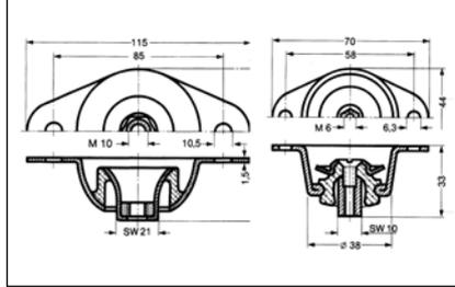
For suspension points, especially those with tensile stress. The elements are protected against breaking off. Natural rubber, optionally in 40° (soft), 55° (average) and 65° (hard) Shore.
