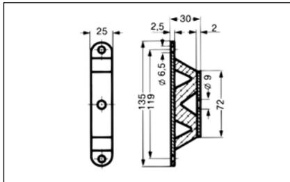
Elastic support of light systems, sensitive instruments and devices. Preferably for compressive and shear stresses.
