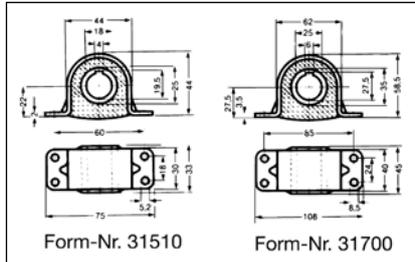
Maintenance-free spherical plain bearings with spring support on all sides with particularly simple mounting. Natural rubber, optionally in 40° (soft), 55° (average) and 65° (hard) Shore.
