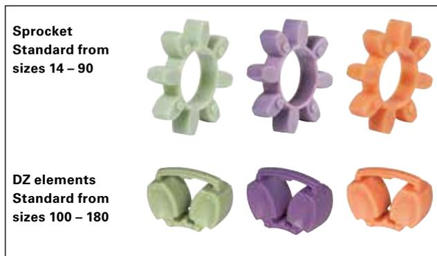
KTR® has developed a new standard material for sprockets. This improved polyurethane, T-PUR, is significantly more temperature-resistant and with longer service life than the previous polyurethane. T-PUR is visually identified by the colours orange (92 Shore A), lilac (98 Shore A) and pale green (64 Shore D). You can of course also continue to obtain the previous polyurethane sockets in the colours yellow, red and natural white with green sprocket marking.
